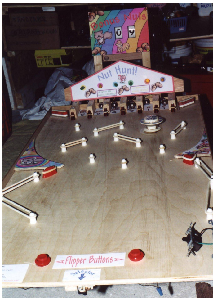
The full Nut Hunt! game. Two top-mounted flipper buttons control the Gottlieb EM flippers at the bottom of the playfield. Player rolls the pinball down the field.
